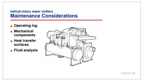
Once a helical-rotary chiller is installed and put into operation, it usually continues to function without a full-time attendant. In many cases, the machine starts and stops on a schedule controlled by the building automation system or a simple time clock. The only daily maintenance requirement is to check the operating log.
